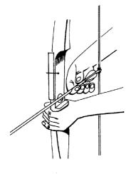
Figure 3: The arrow is set on the string, after (Baier *et al.*, 1976, page 36). The nock is provided with a groove in which the string slightly sticks when the arrow is set on the string. The arrow is supported vertically by the arrow rest fixed to the bow grip and horizontally unilaterally by a pressure button with a built-in spring which is not shown in the figure.
