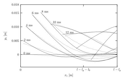
Figure 9: Curves of arrow's deflection on basis of experimental data, dashed line ( --- ) after (Pękalski, 1990), and on basis of new mathematical model for the arrow, solid line ( — ) every 2 ms after release and for model results until arrow nock passes grip. Acceleration force E is predicted force shown in Fig. 7.
