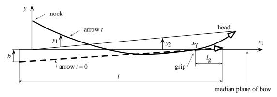
Figure 5: Solid line shows the shape of the arrow, the dashed line is the shape at t = 0, which is out of the median plane of the bow. The displacement out of the median plane is  $y = y_1 + y_2$ .
