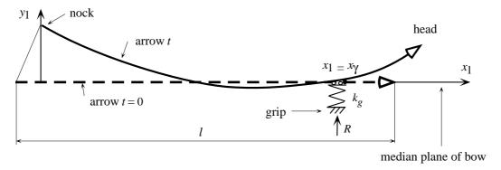
Figure 6: Solid line shows the shape of the arrow when it clears the finger tab. The dashed line shows the shape at t = 0, which is in the median plane of the bow.
