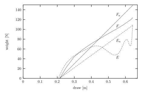
Figure 7: Calculated Static Force Draw curve, F and Dynamic Force Draw curve, E for a modern working-recurve bow. The SFD curve  $F_n$  and the DFD curve,  $E_n$  of the associated linear-spring bow used by Pękalski (1990).
