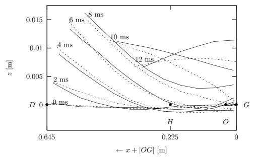
Figure 7: Deformation of arrow: experimental data ( --- ) and calculated by Pękalski ( —— ), every 2 ms after release, [11]. Only parts of the arrow for  $\xi \in [0, \xi_{\gamma}(t)]$  are shown.
