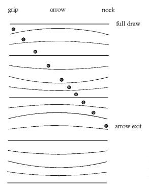
Figure 1: Illustration of archer's paradox (after Klopsteg [3, page 182]). Schematic representation of shapes of arrow during its passage of the bow, based on evidence from speed-flash. photography.
