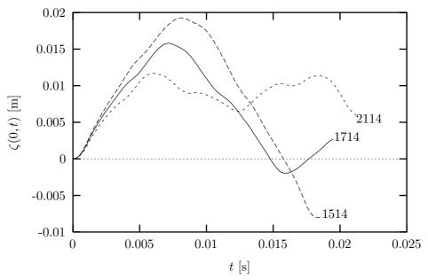
Figure 12: Paths of nock of three different arrows until nock passes pressure point. ( \_\_\_\_ ) standard arrow 1714X7, ( \_\_\_ ) stiffer (and heavier) arrow 2114X7 and ( \_\_\_ ) more flexible (and lighter) arrow 1514X7. Latter arrow slaps against pressure point.
