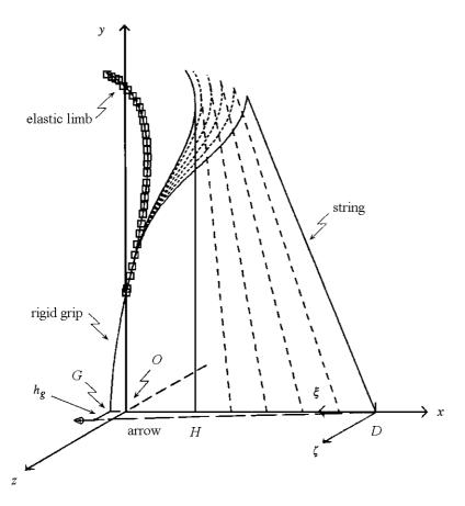
Figure 3: Static deformation of the modern working-recurve bow: the unbraced bow ( $\square$ ), braced bow and fully drawn bow ( — ) and some intermediate situations ( — ). At t=0 the arrow and the moving coordinate system  $(\xi,\zeta)$ , in which the transverse movement of the arrow is described, are shown.
