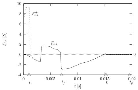
Figure 10: Total force  $F_{tot}$  acting on arrow in  $\zeta$ -direction (13), ( -- ). Also  $F_{tot}^+$ , (14), ( -- ), is shown.  $F_{tot}^+ = F_{tot}$  for  $t > t_r$ . Arrow looses contact with pressure point definitely at  $t = t_f$ . Arrow leaves string at  $t = t_l$  and nock passes pressure point at  $t = t_g$ .
