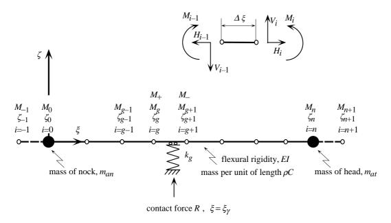
Figure 6: Scheme of model of arrow. Each element,  $i=1,\cdots,n$ , has length  $\Delta \xi$ . Between grid-points we have mass per unit of length  $\rho C$  and flexural rigidity EI. Two fictitious points outside arrow are introduced, grid-points i=-1 and i=n+1. Pressure point at  $\xi=\xi_{\gamma}$ . Grid point to the left of pressure point is denoted by g. Two extra unknown bending moments  $M_{-}$  and  $M_{+}$  at points g and g+1, respectively.
